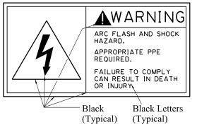
The switchboard, all enclosures, disconnects, junction boxes, etc. that contain service voltage of 120/240 shall have one or more labels with  $\frac{1}{2}$  in. high (minimum) letters and shall read as follows:
